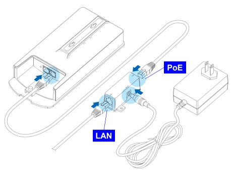
Figure 2-1: Installing the ENS202
