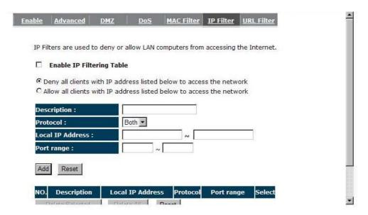
**Enable IP Filtering:** Check to enable or uncheck to disable IP Filtering.
