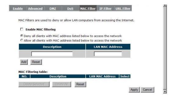
**Enable MAC Filtering:** Check to enable or disable MAC Filtering.
