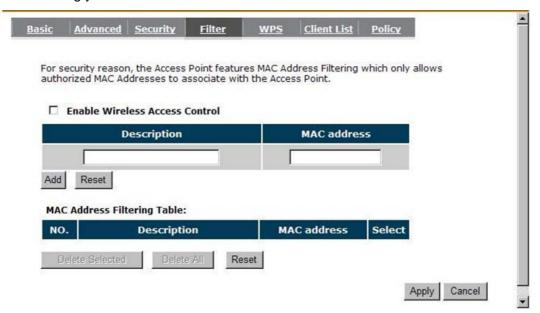
Enable wireless access control: Enable the wireless access control function
