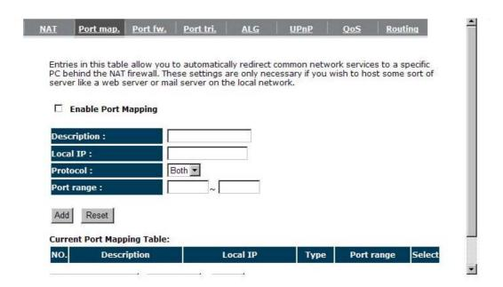
**Enable Port Mapping:** Enable or disable port mapping function.
