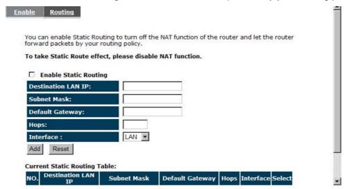
**Destination LAN IP:** Specify the destination LAN IP address of static routing rule.
