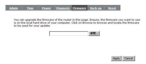
Once you've selected the new firmware file, click < Apply> at the bottom of the screen to start the upgrade process
