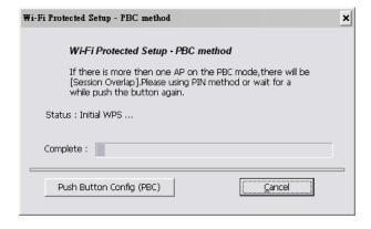
Press WPS Button on USB directly and then click the button "**Push Button Config**" shown above.
